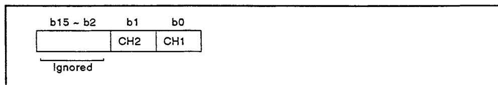
Fig. 3.7 Analog Output Enable/Disable Channel Area Data Map
